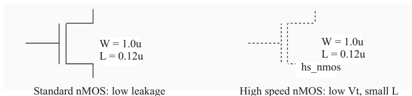
Fig. 3.36 The low leakage MOS symbol (left) and the high speed MOS symbol (right) (MosOptions.SCH)
