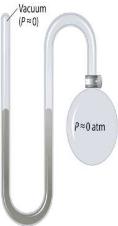
(a) Closed-end manometer
