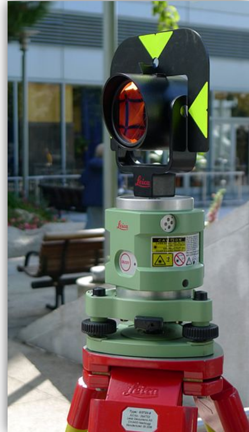
“Round prism and laser plummet on tripod” , by KJG2007 available under CC BY-SA 2.0
