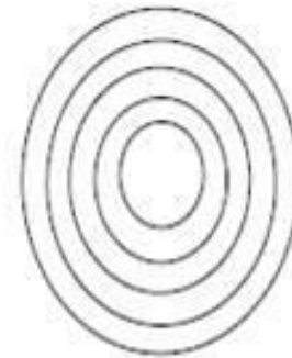
(b) Track pattern on a magnetic disk
