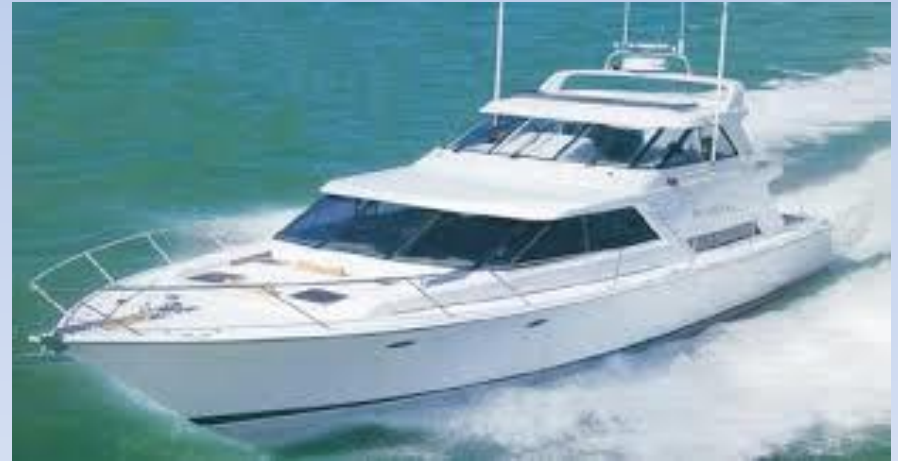
www.yanmarhelp.com Planing hull : a hull designed to climb up and sit on the bow wave as it moves forward.
