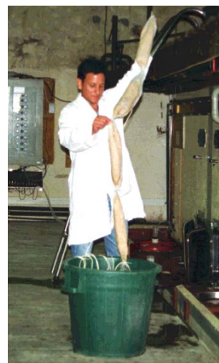
Figure 4. The encapsulated yeasts are placed in Nylon bags, which length has been adapted to the fermentation vat height. A ballast is fixed at the inferior extremity of the bags in order to avoid them from floating. The bags are hung up to the superior part of the fermentation vat (A). Before being introduced into the fermentation vat, the bags containing the balls are rehydrated during 30 minutes in a solution sugared with 40g/L of saccharose in order to reactivate the yeasts (B)
