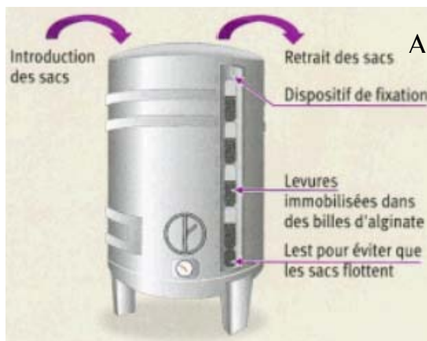
Figure 4. The encapsulated yeasts are placed in Nylon bags, which length has been adapted to the fermentation vat height. A ballast is fixed at the inferior extremity of the bags in order to avoid them from floating. The bags are hung up to the superior part of the fermentation vat (A). Before being introduced into the fermentation vat, the bags containing the balls are rehydrated during 30 minutes in a solution sugared with 40g/L of saccharose in order to reactivate the yeasts (B)
