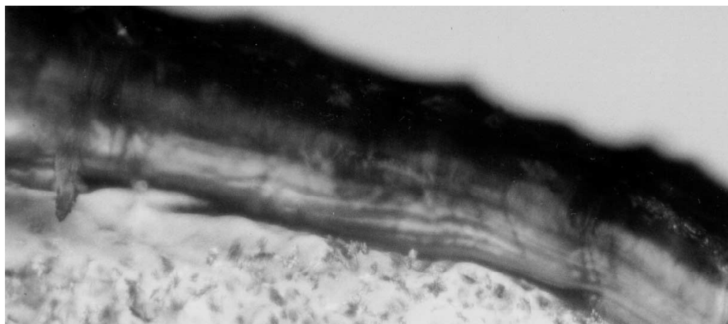
Fig. 17. Micrograph of the frontier area between surface and middle layer within a cellulose pellicle loaded with \text{CoSO}_4 (original magnification 3.2\times ).
