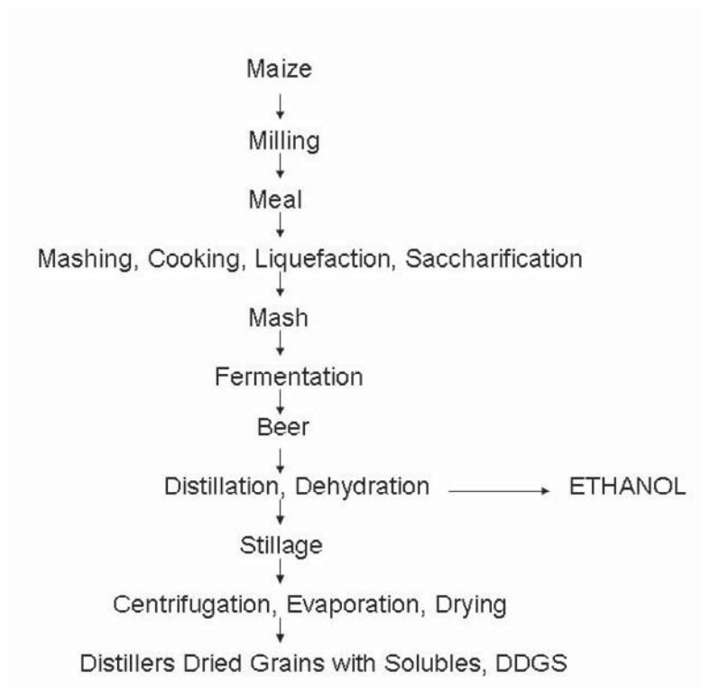
Fig 4.5 Ethanol production from maize (dry-grind process)
