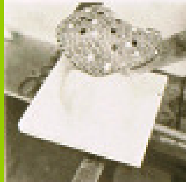
44 Stamping. While still hot, the disc is dropped over a ceramic form made in the shape of the final object, in this case a semi-spherical bowl.
