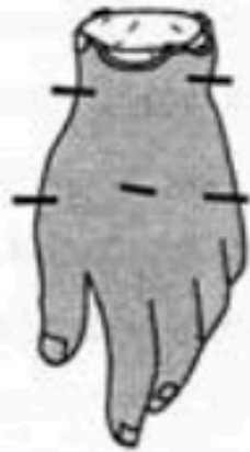
5. Finished wax working model with fingernails marked, clay core poured inside, and metal chaplets stuck through wax into core.
