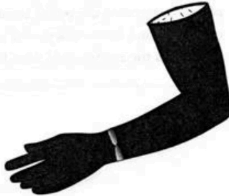
10. Hand joined to arm by flow weld.
