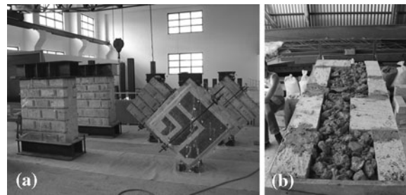
Fig. 1 a Three-leaf stone masonry wallettes, simulating the masonry of the Katholikon of Dafni Monastery and b the infill material
