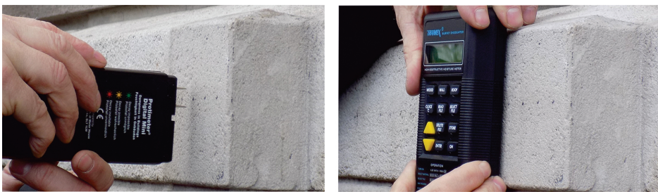
Figure 6. Left: Pin moisture meter (Profimeter), right: pinless moisture meter (Tramex).
