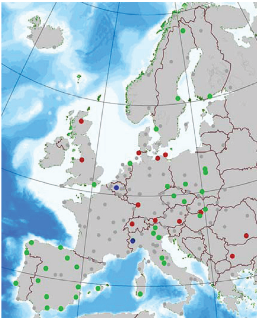
Fig. 2 EPN stations delivering real-time data: RTCM – green; raw data – red; RTIGS – blue
