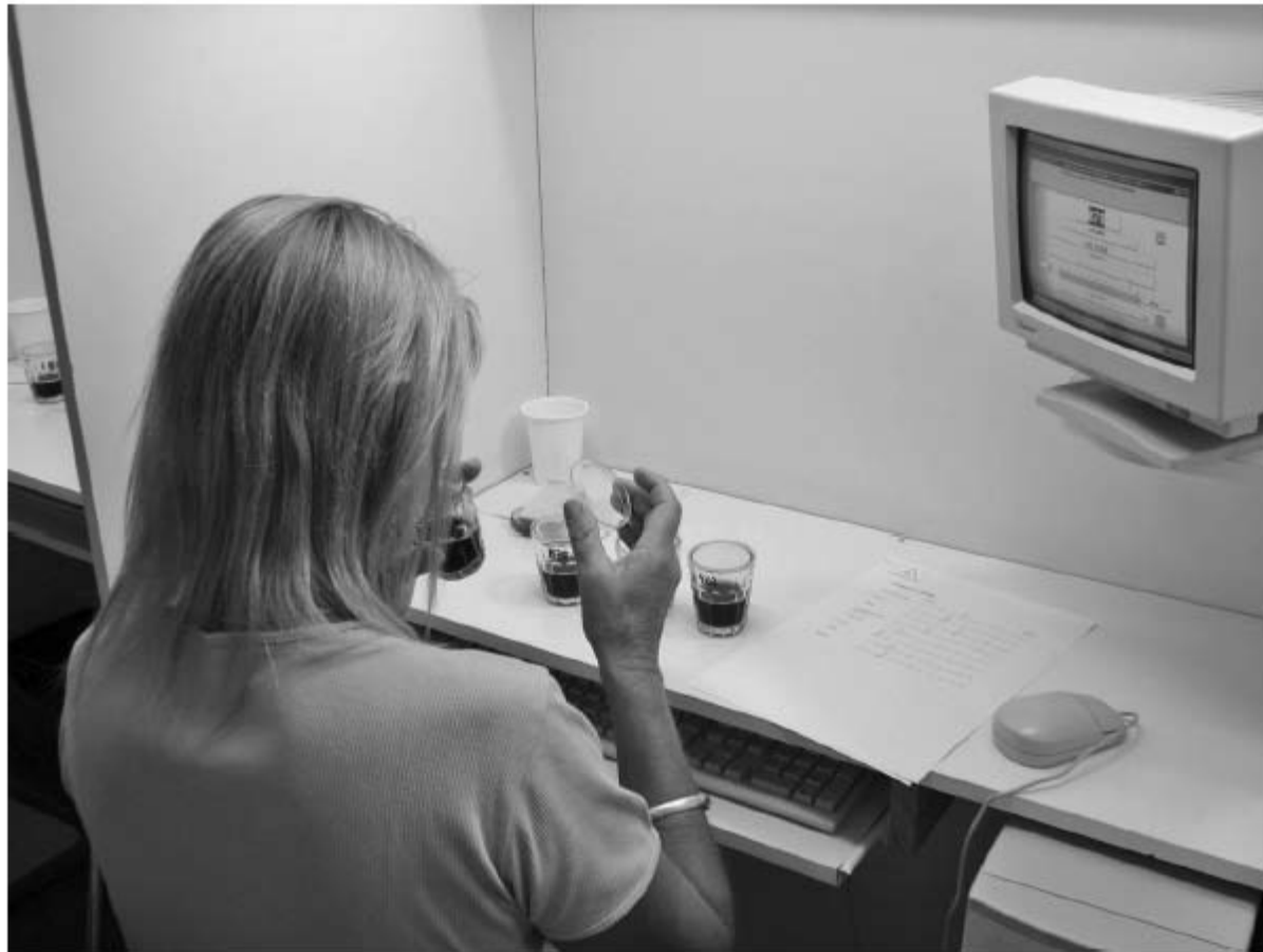
Figure 2.2 Trained assessor measuring the aroma of a beverage in a sensory laboratory equipped with individual booths and a computerized data acquisition system.
